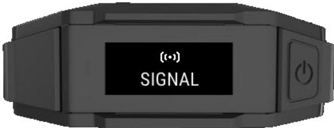
If the camera is in the buffering mode and a signal event occurs, the camera will begin recording
