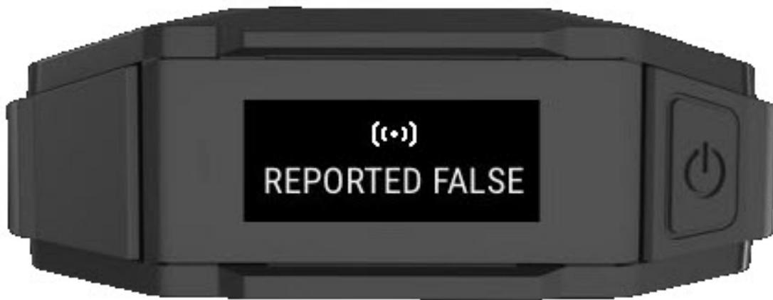
Press the Select button, the signal activation will be reported false, the camera will end the recording, and return to buffering mode
