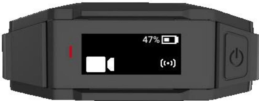
If the Select button is not pressed within 10 seconds, the message is removed, and the camera will continue recording
